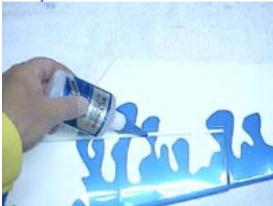
#2 Start by centering all the CA hinges in slots and applying thin CA (Do not use kicker on hinges)
